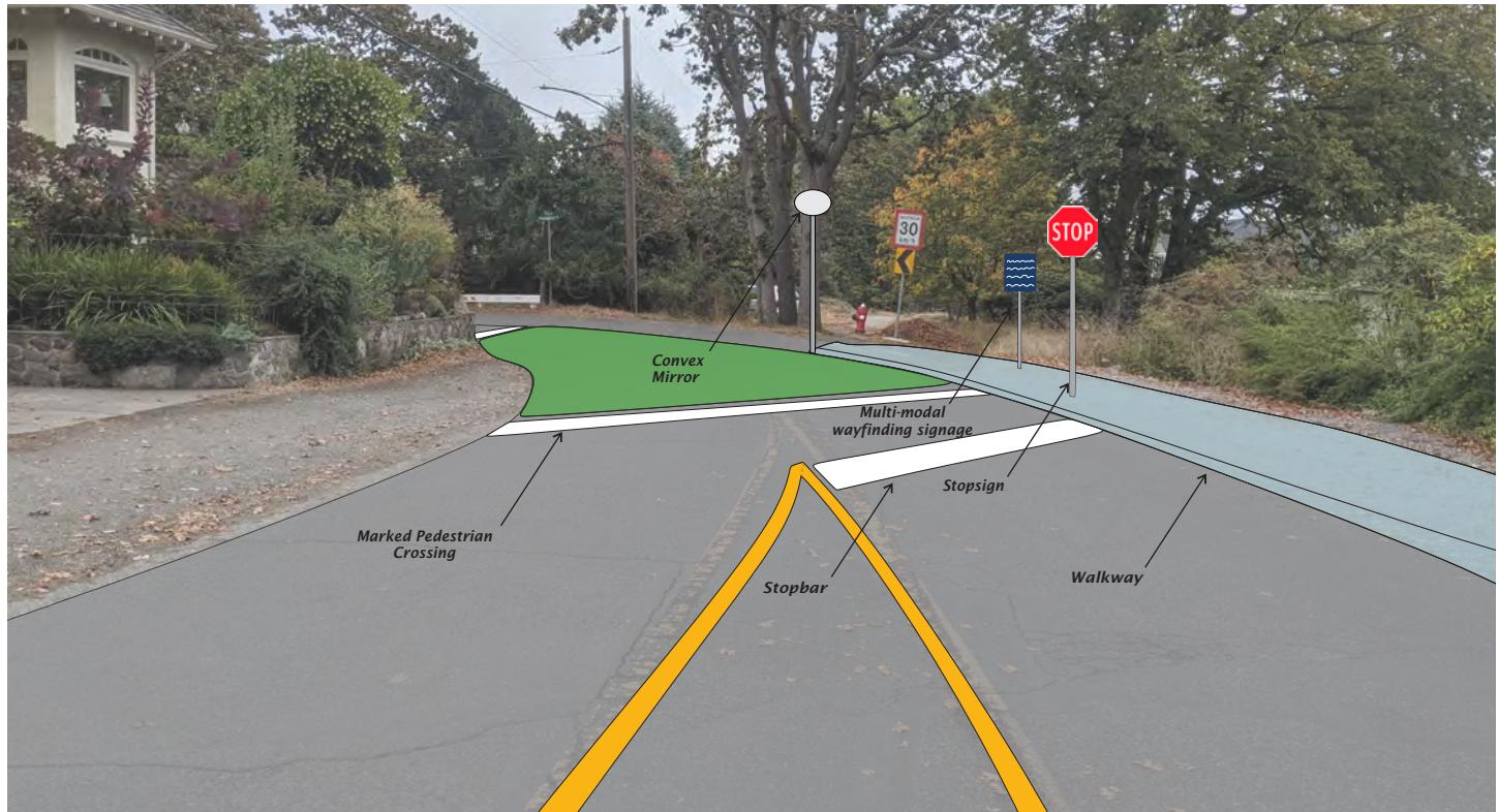
**Figures 7.3, and 7.4** show the views in the opposite direction. This is an example of a corner that could benefit from the following design measures to slow vehicle speeds and improve pedestrian visibility and presence:
