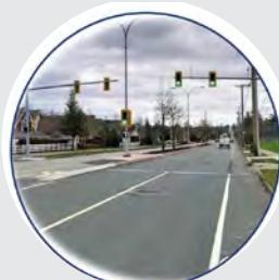
**Pedestrian activated signals** are full traffic signals that stop vehicles and pedestrian when activated by a push-button.
