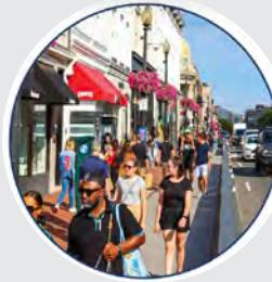
**Widened sidewalks** narrow the roadway, reduce vehicle speeds, and provide more accessible manoeuvring space for pedestrians.
