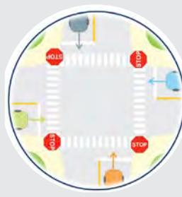
**All-way stop controls** force vehicles to stop at each leg of an intersection, as opposed to a two-way stop control, which allows vehicles to travel freely along the higher volume street.
